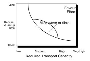
This demonstrates the relationship between "Required Transport Capacity" and "Turn-up Time" for microwave and fibre applications. Microwave is favoured for quick turn-up, low, medium, and high
