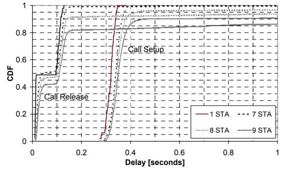
Fig. 6. CDF for the call setup and call release delays with the 11 Mbit/s transmission rate.
