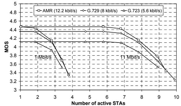
Fig. 10. Downlink average MOS for three low bit rate codecs at 1 Mbit/s and 11 Mbit/s.
