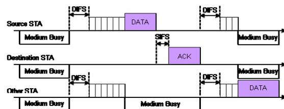
Fig. 1. Basic Access mechanism.
