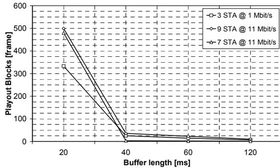
Fig. 8. Downlink average playout blocks versus the dejittering buffer length.
