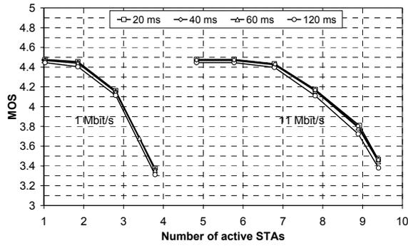
Fig. 7. Downlink average MOS for different dejittering buffer lengths with the transmission rates of 1 Mbit/s and 11 Mbit/s.
