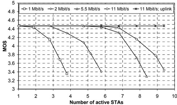
Fig. 5. Downlink average MOS for the IEEE 802.11b transmission rates and uplink MOS for the 11 Mbit/s rate.
