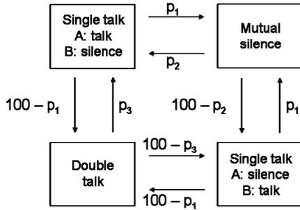
Fig. 2. State transition model for a conversation.
