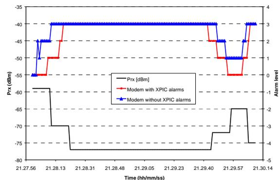
Fig. 5: Received power and alarm levels during rain fading event on 23rd of May.
