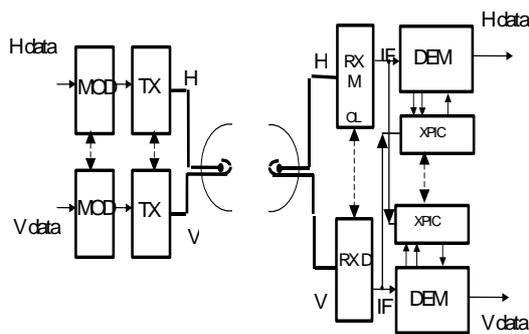
Fig. 1: Typical XPIC architecture.
