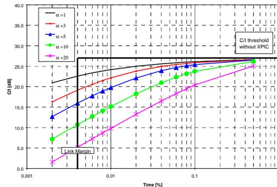
Fig. 9: C/I ratio for different rain fading and rainfall inclination ( $\alpha$ ).
