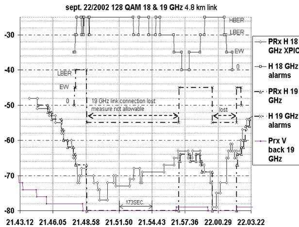
Fig. 8: Received power and alarm levels during rain fading event on 22<sup>nd</sup> of September.
