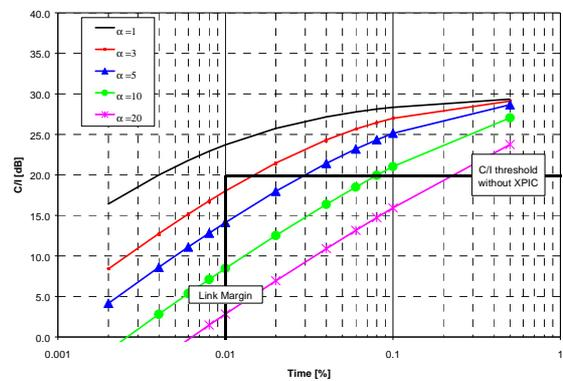
Fig. 8: C/I ratio for different rain fading and rainfall inclination ( $\alpha$ ).
