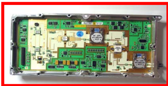
Fig. 4: Power Amplifier Unit
