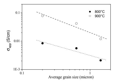
Influence of the average grain size on the apparent ionic conductivity of La<sub>0.5</sub>Sr<sub>0.5</sub>FeO<sub>3-δ</sub>
