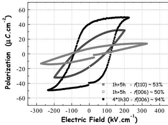
**Figure 3** Hysteresis loops versus film orientation and deposition procedure of  $\text{LiNbO}_3$  thin films sputtered onto ITO-covered  $\langle 111 \rangle$ -Si. Films of Figures 1 and 2. Applied field ( $E_a$ ):  $120 \text{ kV}\cdot\text{mm}^{-1}$ ; 100Hz
