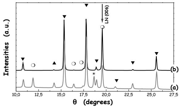
**Figure 1** X-ray diffraction patterns of LiNbO<sub>3</sub> thin films sputtered onto ITO-covered <111>-Si substrates and annealed in air at 750°C for 1h **(a)** 1h/600°C + 5h/600°C **(b)** four steps, 3\*1h30/300°C + 1\*1h30/600°C The relative intensity of LN (006) peak increases for multi-layered structures. Parasitic phases can be suppressed in as-deposited composite systems.
