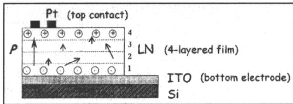
**Figure 4** Schematic representation of a 4-layered LN film deposited onto ITO-covered  $\langle 111 \rangle$ -Si.
