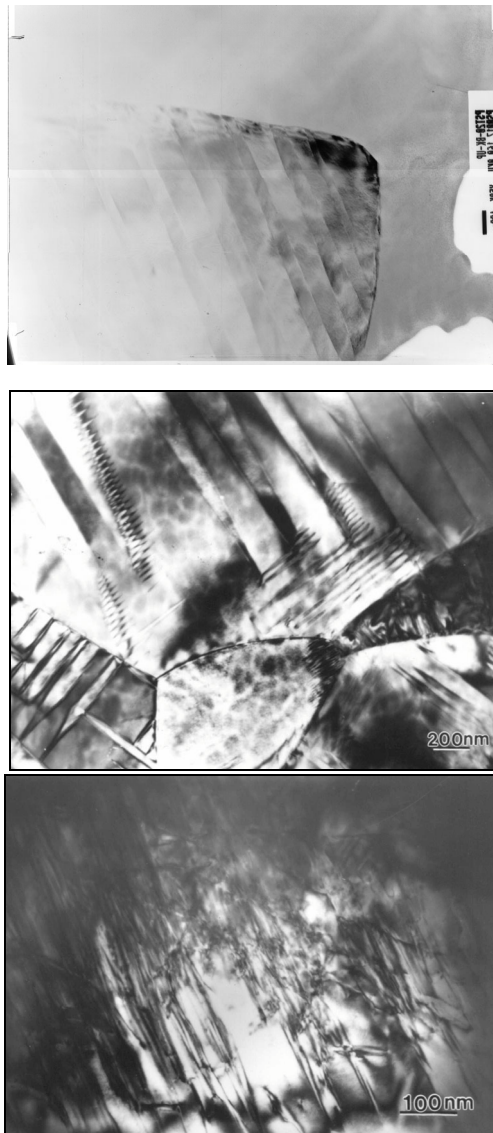
Figure 2 TEM micrographs showing microstructural evolution of \text{Pb}_{0.6}\text{Sr}_{0.4}\text{TiO}_3 ceramics under polarization switching at a working frequency of 1 kHz and 55 kV/cm. (a) as-sintered state; (b) polarization switching for 10^5 cycles; (c) 3 \times 10^9 switching cycles.
