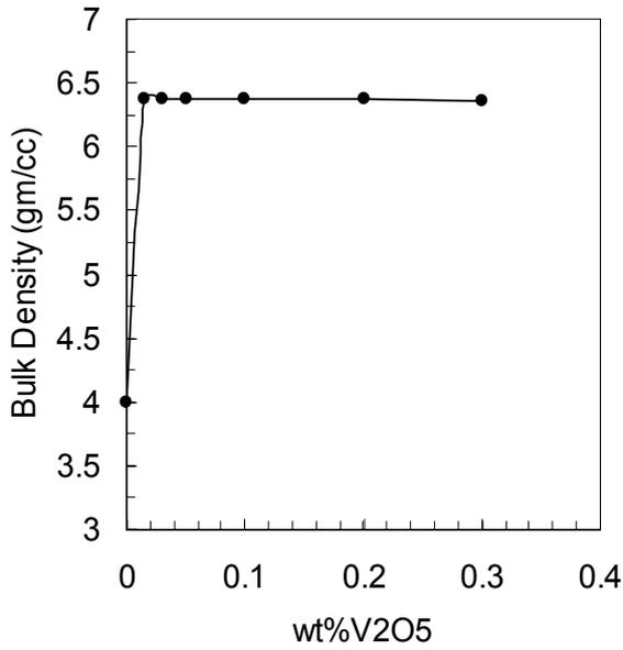
Figure 1. Bulk densities of BCZN ceramics as a function of  $V_2O_5$  content.
