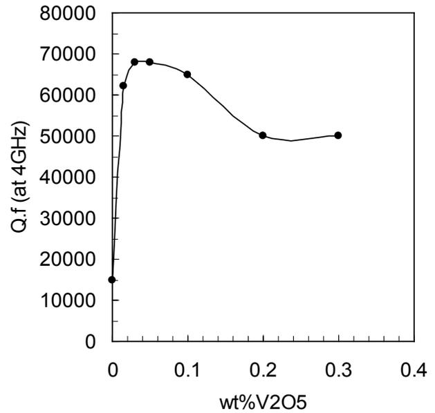
Figure 2. Q.f values of BCZN ceramics as a function of  $V_2O_5$  content.
