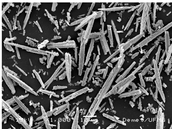
FIG. 2. Scanning electron micrograph of a BMN sample (magnification of 1,000 \times ) obtained by microwave-assisted hydrothermal processing at 200 °C for 2 h. The scale of the figure is 125 \mu\text{m} \times 95 \mu\text{m} .
