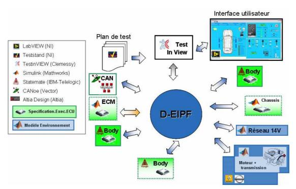
The validation is done by gathering all the runnable specifications of each ECU from the different departments (chassis, body, engine...) and simulating them together including environment models (electrical distribution, vehicle dynamic...). The CAN network is also simulated in order to be predictive in terms of communication.
