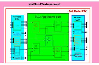
• **Part ECU model**: it is a simple representation of the behavior of the ECU but it is not the specification itself. It is used to replace the ECU specification.
