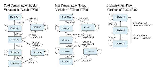
Note:  $\Delta$ HeatSource>0 (resp. < 0) means an increasing (resp. decreasing) of heat source. Thus we finally obtain a set of paths containing all potential behaviors. The following picture describes one of them
