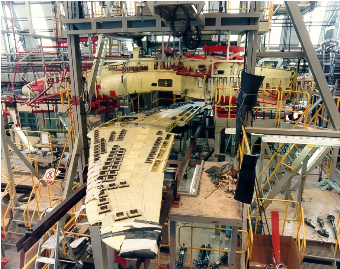
Figure 4 - The Hawk Life Extension Fatigue Test (LEFT)
