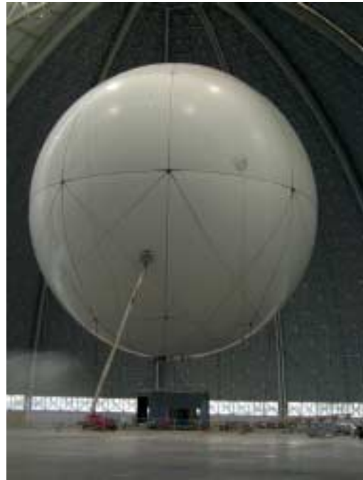
Fig. 4 Side view of the CL 75 Airplane during integration, diameter of the envelope is 60m
