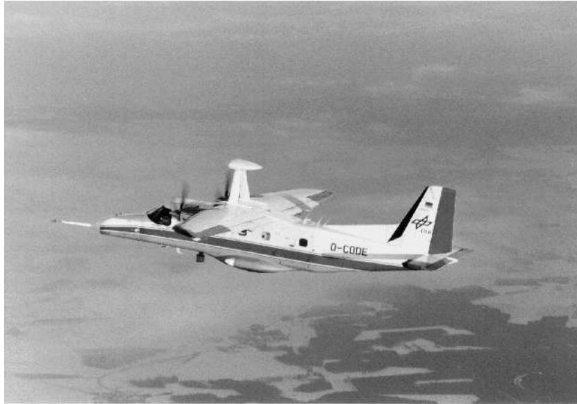
Figure 2. The HiVision sensor from DASA, Ulm on DLR's DO 228. It is an imaging FMCW radar with center frequency of 35 GHz, field of view of 41^\circ/3.5 km, RF output 0.5 W, azimuth resolution 0.25^\circ per pixel, range resolution 6.67m per pixel, vertical beam width about 10.0^\circ and a frame update rate of about 15 Hz.
