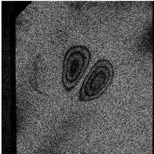
Fig. 12 Examples of Laser-Shearographic Measurements, strain deviation indicates a delamination in a C/SiC panels (courtesy DLR,Stuttgart)
