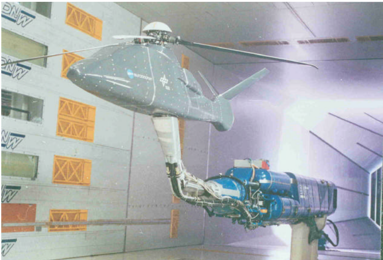
Fig. 2 : Wind tunnel testing in DNW
