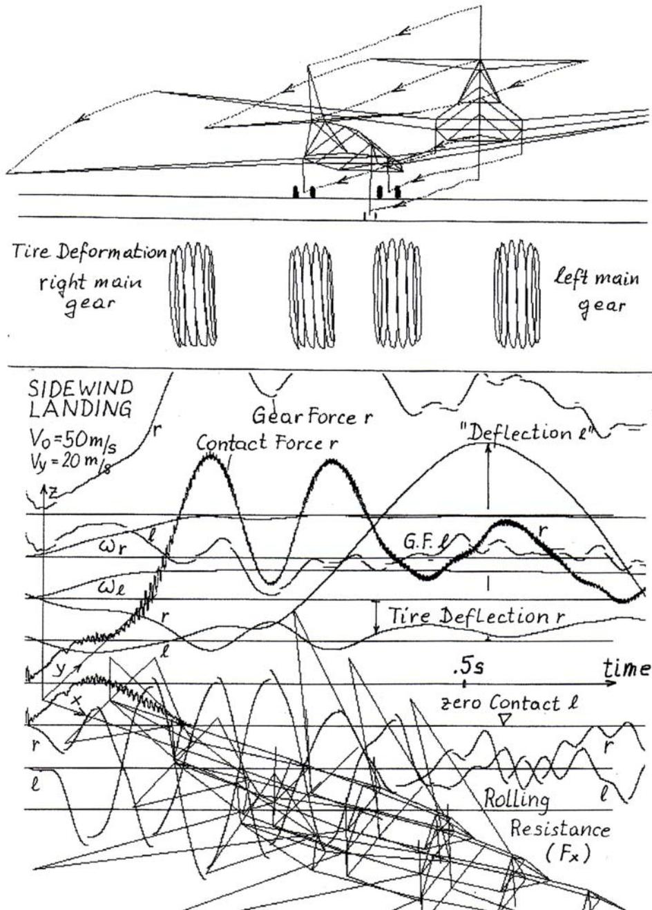
Fig 10: Side-Wind landing of 72 km/h when landing velocity is 180 km/h is a strong demand of the gears by shifting the vertical forces to one side and also the horizontal forces producing a gear-walk. The longitudinal forces have amplitudes bigger than 20 to.
