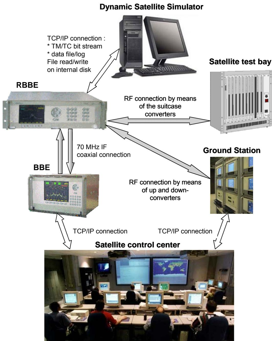
**Figure 3 : multiple missions for the satellite simulator**
