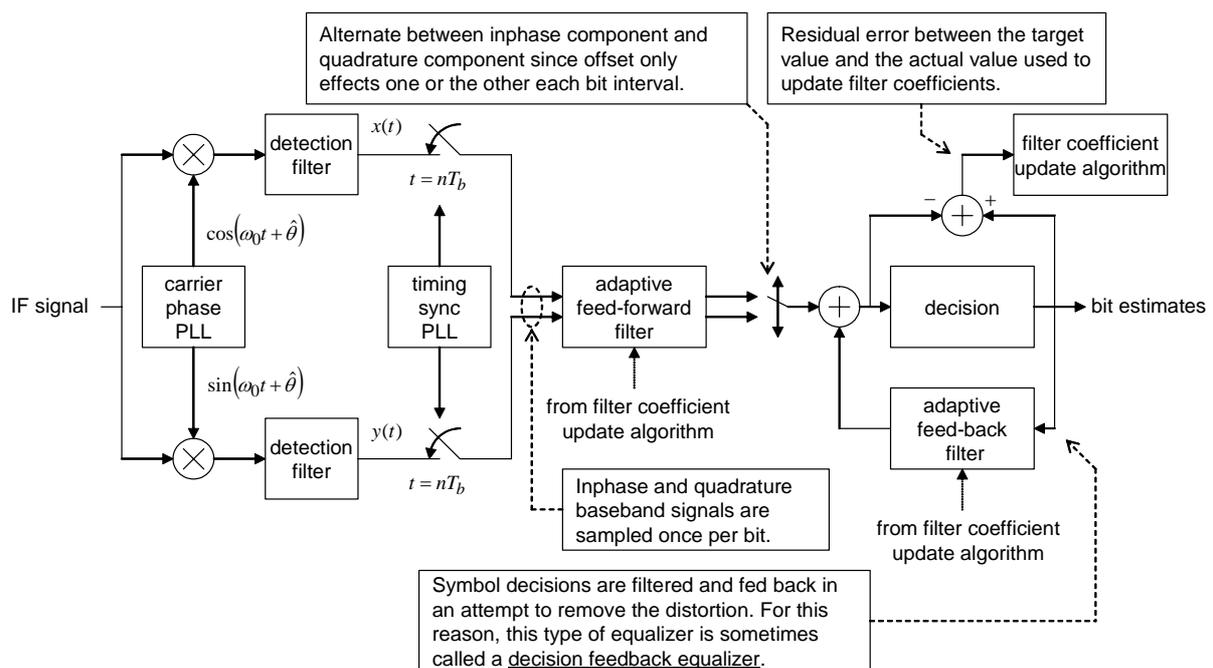
Figure 6: Block diagram of the adaptive decision feedback MMSE equalizer for SOQPSK.
