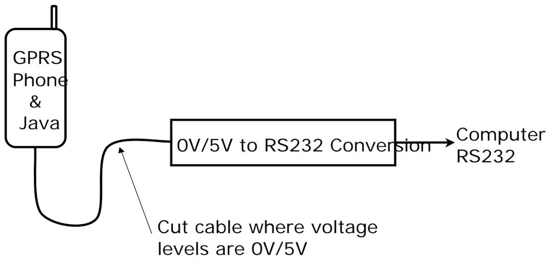
**Figure 2. GPRS Phone-to-Computer Serial Interface Cable with In-Cable Voltage Conversion**
