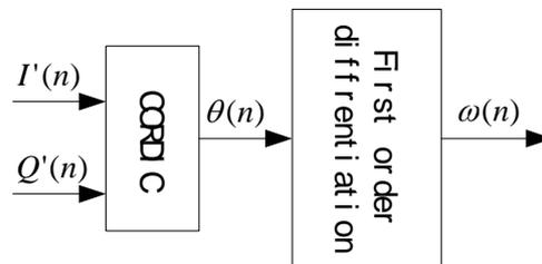
Fig.4 Structure of frequency discriminator
