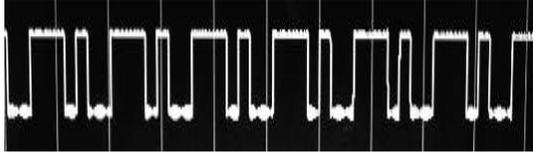
Fig.11 Output when PCM/FM level is -50dBm
