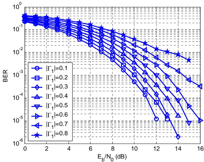
Figure 9: Bit error rate performance of 20 Mbit/sec SOQPSK-TG in the multipath channel with impulse response (15) with equalization. The equalizer consisted of 21 feed forward coefficients, 18 feedback coefficients and used a step size of 0.001. Compare with Figure 10.
