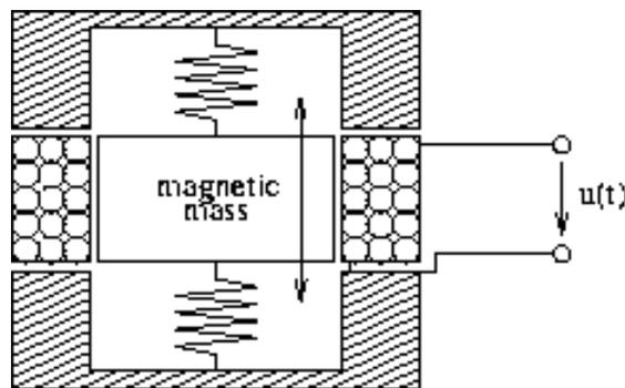
Fig. 4 Design Principle of a Geophone
