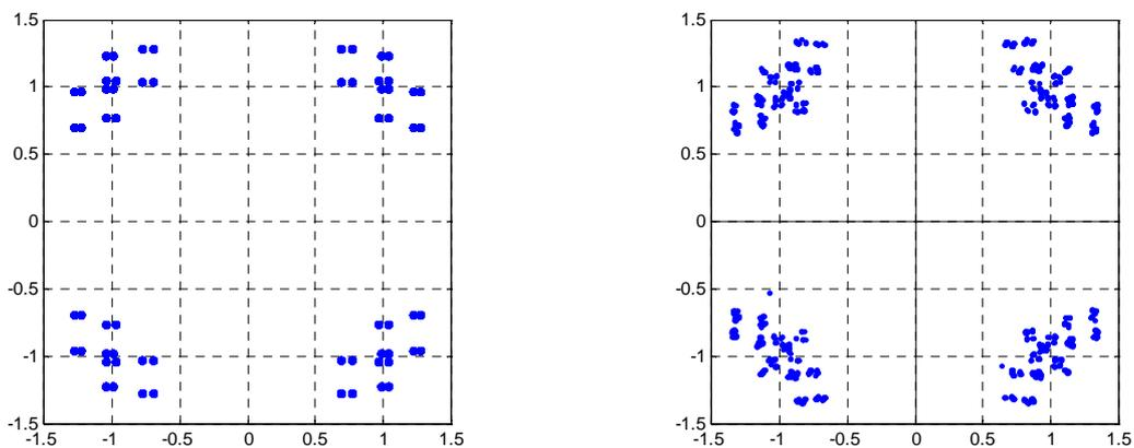
Figure 3: I/Q decision points for FQPSK (left) and SOQPSK-TG (right) using an integrate and dump detection filter in a noiseless environment.
