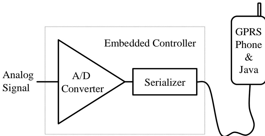
Figure 1. Basic Components of GPRS Phone-based Analog Measurement
