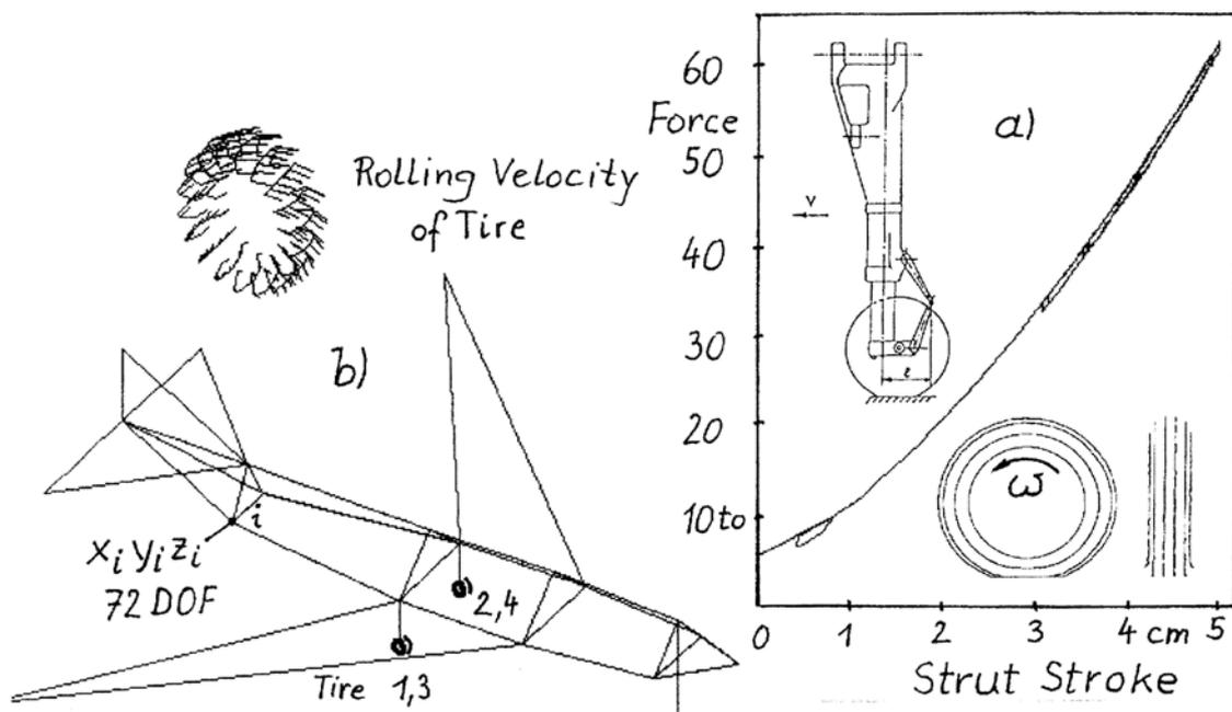
Fig 6 a) The strut force is nonlinear and belongs to the maximum loaded main gear of Fig 10 example.
