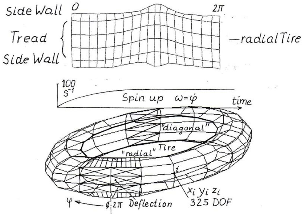
Fig. 1 For conventional (diagonal) tire sidewall and tread are enforced by cables which are crossing in several layers with the same angle, for radial tires the cables in sidewall are not crossing but in tread they are laying in three crossing layers. The computer model is only a rough numerical net for fast computation but the used parameters correspond to the continuum theory of infinite fine nets [6]. On top lateral deformation is drawn.
