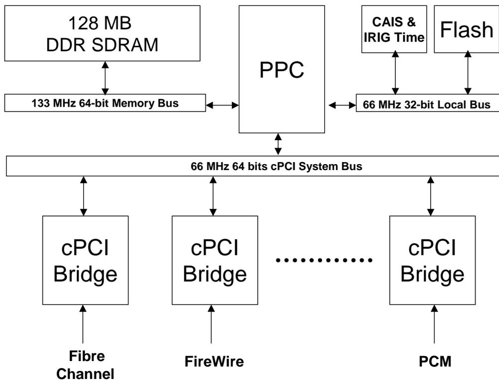
**Backplane:** A CompactPCI Bus-like backplane was chosen as the backbone of the unit. The backplane operates with 64-bit wide at 66 MHz operating rate using up to four I/O slots. This translates to a peak bandwidth of 528 megabytes per second (MB/s). Accounting for protocol overhead, bandwidth of over 200 MB/s is realizable within the multiplexer. Several signals were added to the backplane bus to meet IRIG-106 Chapter 10 time tag requirements, and other miscellaneous signals.
