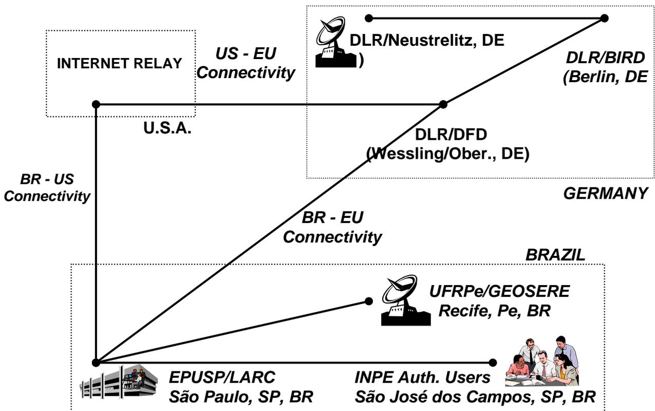
**Figure 1 - Backbone Topology of the Information Networks**
