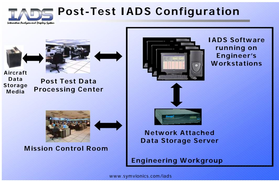
Figure 2. The Post Test IADS System Architecture
