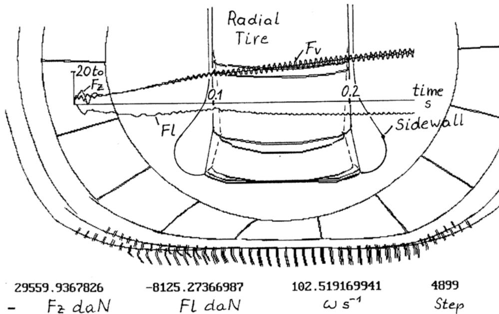
Fig.3 The radial tire is computed under the same conditions than the conventional tire. It isn't vertical so stiff but has a better grip and fewer abrasion.
