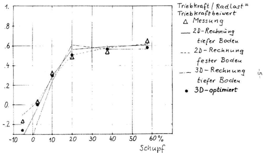
Fig. 5 Measurement and computed of traction characteristics on deep ground channel at TU Munich
