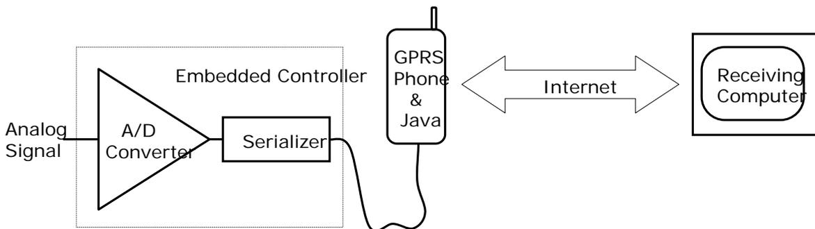
**Figure 3. Conversion of Analog Signals, Transmission to GPRS Phone via Serial Cable, Transmission to Destination Computer via Internet.**
