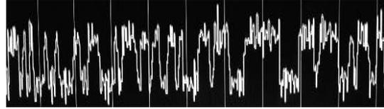
Fig.12 Output when PCM/FM level is -1dBm
