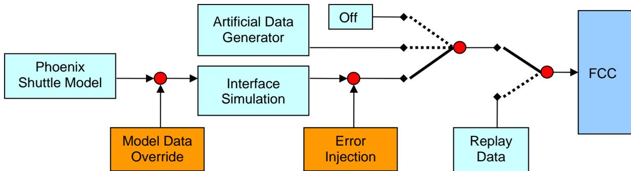
Fig. 7: Data Flow of Sensor Signals in SAS
