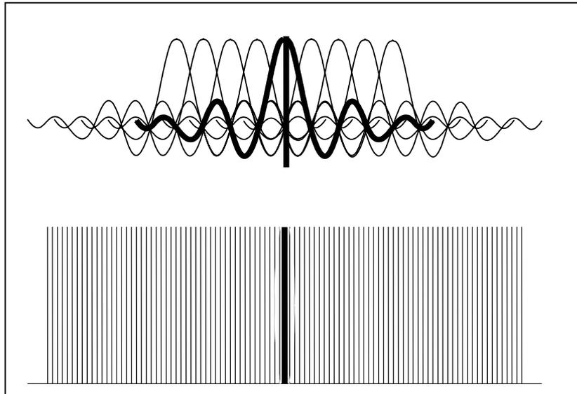
Fig. 4. The Relationship of RF Carriers in COFDM
