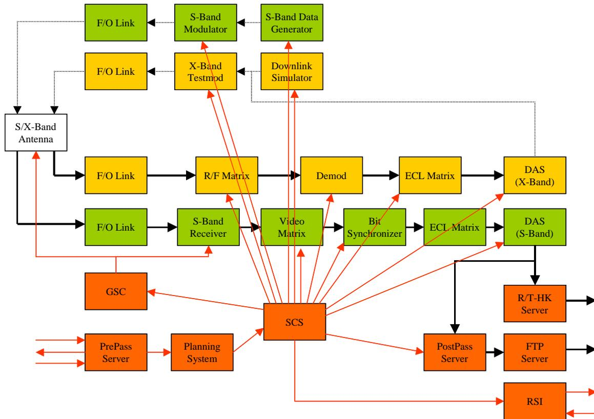
**Figure Overview of all components used for TerraSAR-X data reception at the ground station Neustrelitz (F/O-link: fibre optic link; SCS: Station Control System; GSC: Ground station Controller, RSI: Receiving Station Interface ; DAS: Direct Archive System)**
