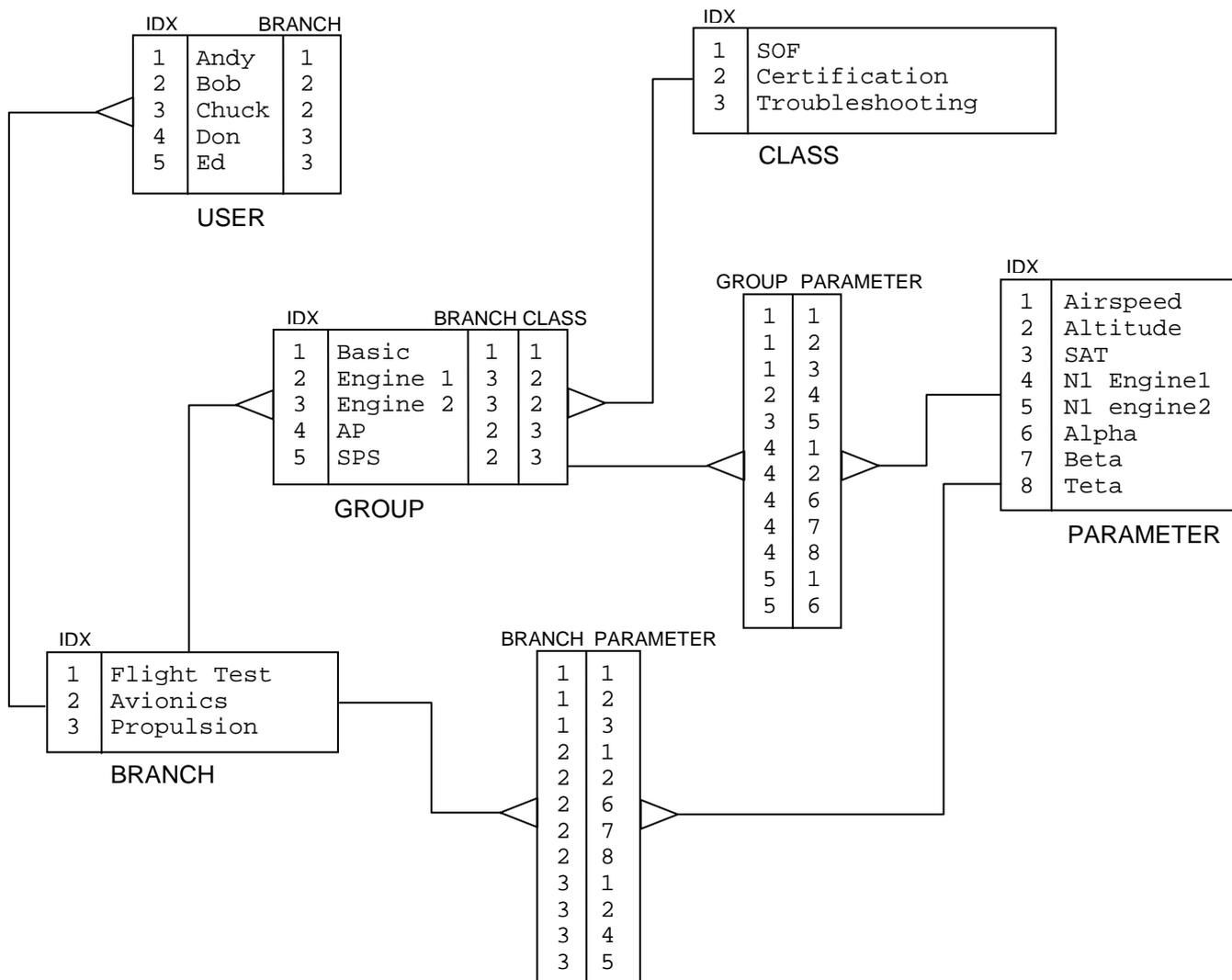
Figure 1 – Proposed Data Model for Parameter List Management
