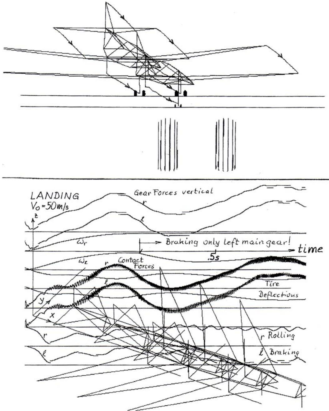
Fig. 9 In this computation the influence of non symmetric braking is documented. The deviation from straight run is very small, but by longer computer run may be of interest.
