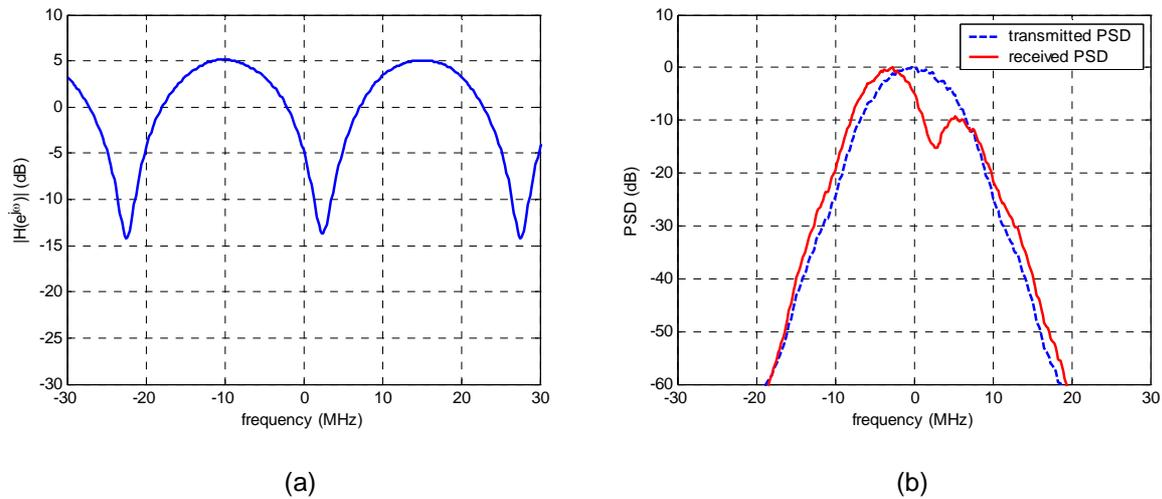
Figure 4: Frequency selective multipath commonly found in aeronautical telemetry. (a) Channel transfer function of corresponding to the impulse channel impulse response (7). (b) The effect of this channel on the spectrum of 20 Mbit/sec SOQPSK-TG.
