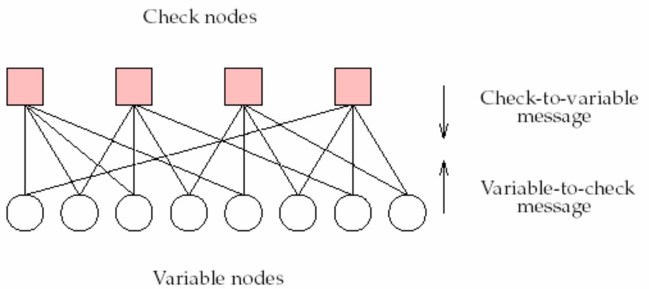
FIGURE 1. Trellis representation of an LDPC code
