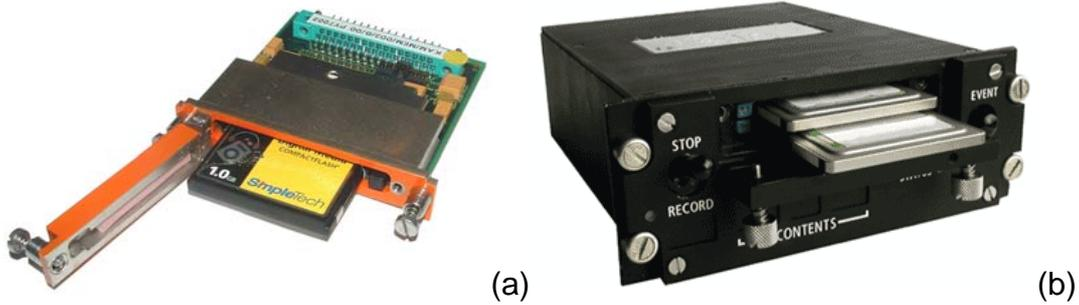
Figure 4 - (a) CF based DAU recorder (b) PC card Cockpit recorder
