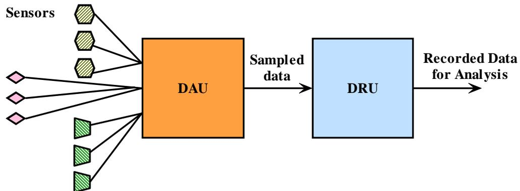
*Figure 1 - Overview of a basic OLM system*
