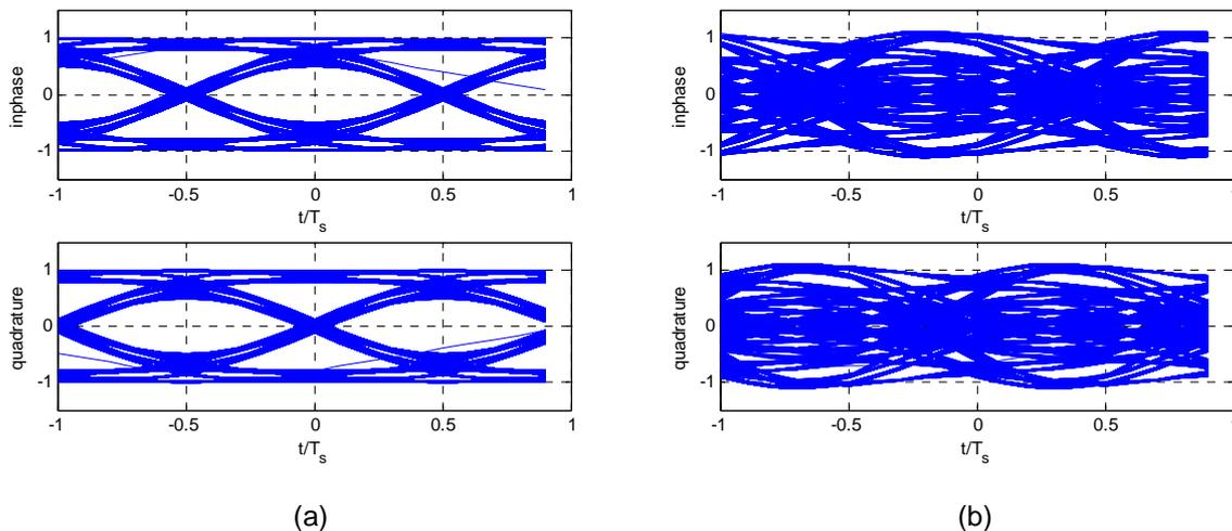
Figure 5: Eye diagrams for SOQPSK-TG using a simple integrator for the detection filter. (a) The eye diagram for the case of no multipath. (b) The eye diagram for the case of multipath interference given by the channel impulse response (7).
