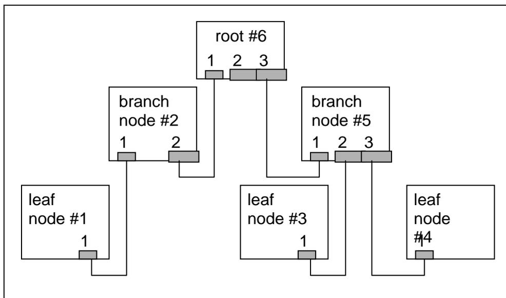
**Figure 1: Example of a FireWire Topology**
