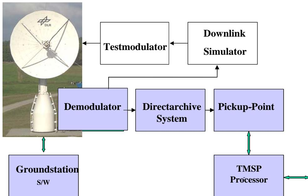
Figure 2: Overview about the TerraSAR-X components for the reception of the X-Band-downlink
