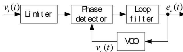
Fig.1 Model of phase locked demodulator
