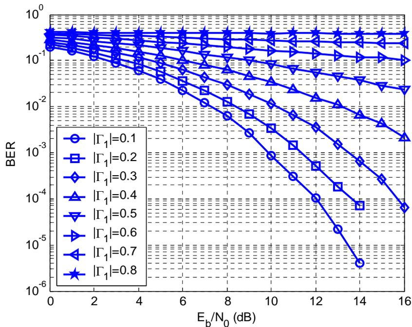
Figure 10: Bit error rate performance of unequalized 20 Mbit/sec SOQPSK-TG in the multipath channel with impulse response (15). Compare with Figure 9.
