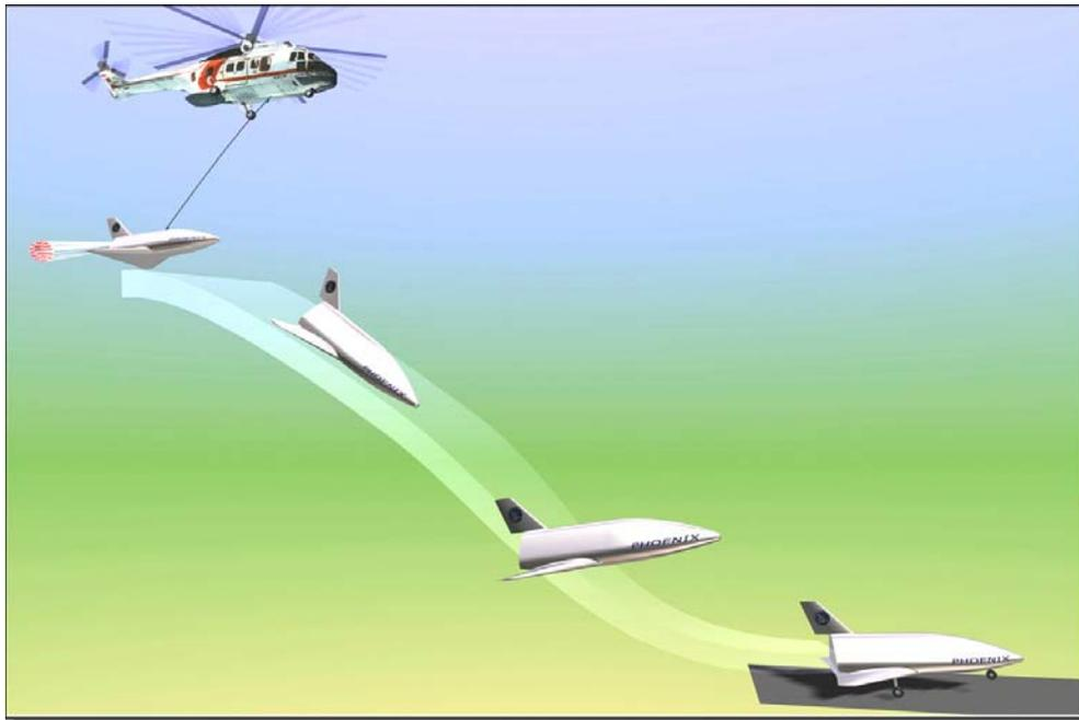
*Fig. 2: Helicopter Drop Test using Phoenix*
