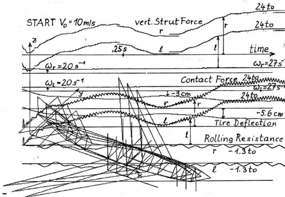
Fig 7 At first the tire is in air but is expanding by inner pressure acting. Then it touch the ground and gets a vertical impulse. It looses again contact and develop a rough linear increasing contact force. The strut force comes down from  $-5.5\text{ to}$  prestress and then increases also. The tire deflection is only the mean value - of axle high minus nominal tire radius of  $50\text{ cm}$  which increases by inner pressure for  $\sim 1\text{ cm}$ . Contact forces are drawn for two tires.
