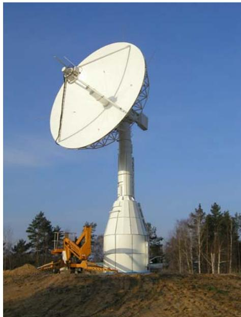
Figure 3 S/X-band ground station antenna at DLR-DFD Neustrelitz
