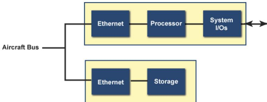
**Figure 4 Storage in a distributed system**
