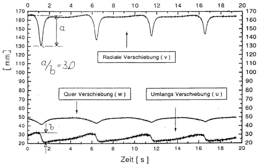
Fig.4 Measurements of non stationary deformations of an equator point of a tire AS 18.9 R 34 on the flat bed test rig at TU Berlin.
