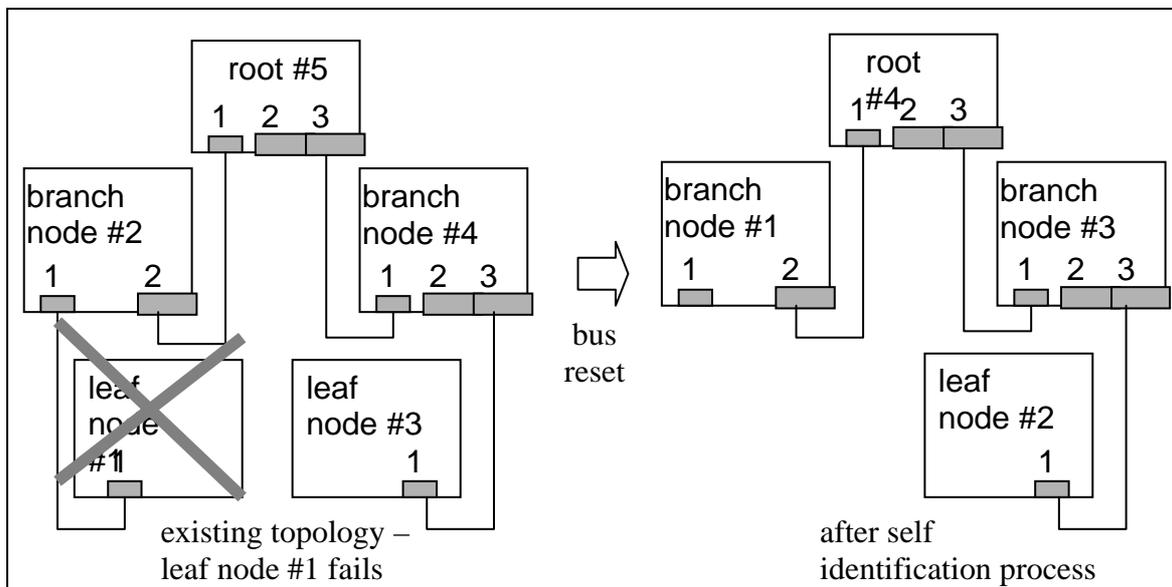
**Figure 3: Dynamic Assignment of Physical IDs on the FireWire Bus**
