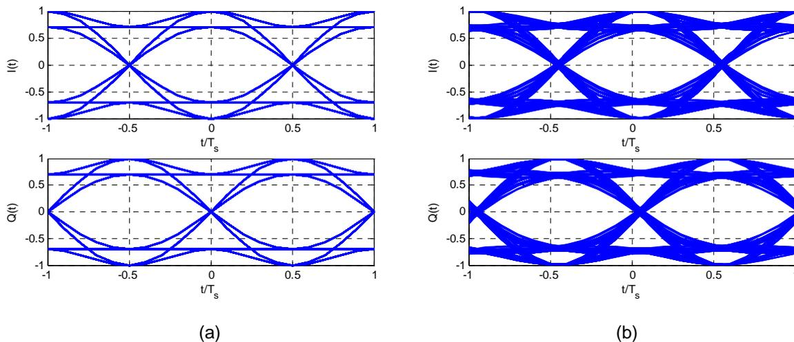
**Figure 1: Eye diagrams for the inphase and quadrature components of FQPSK (a) and SOQPSK-TG (b).**
