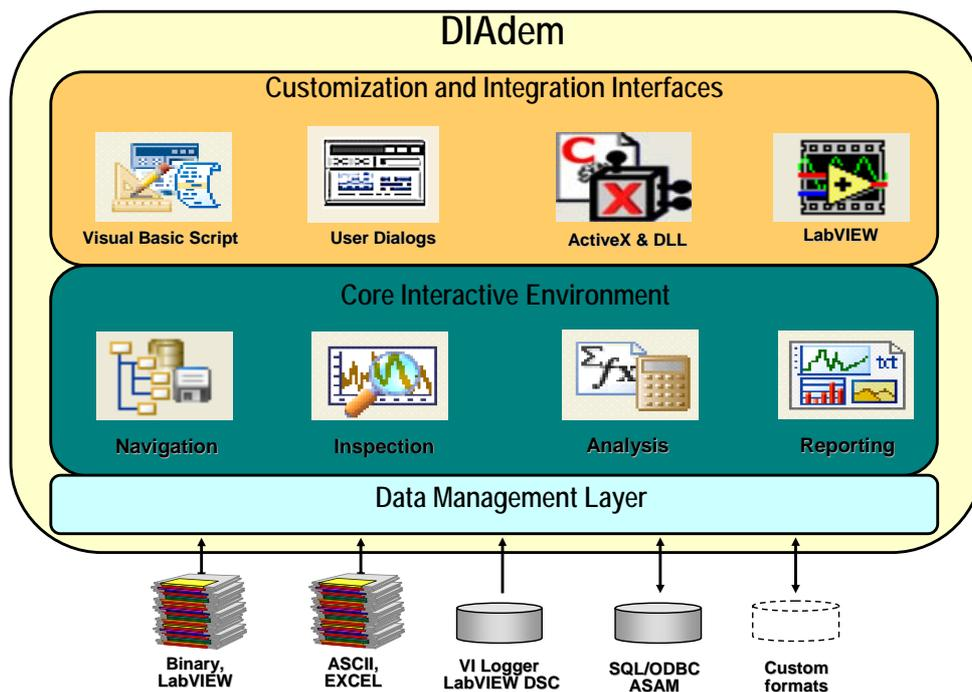
**Figure 3: DIAdem combines functionality for analysis and report generation while also providing an open data interface as well as comprehensive features for automating repetitive tasks**
