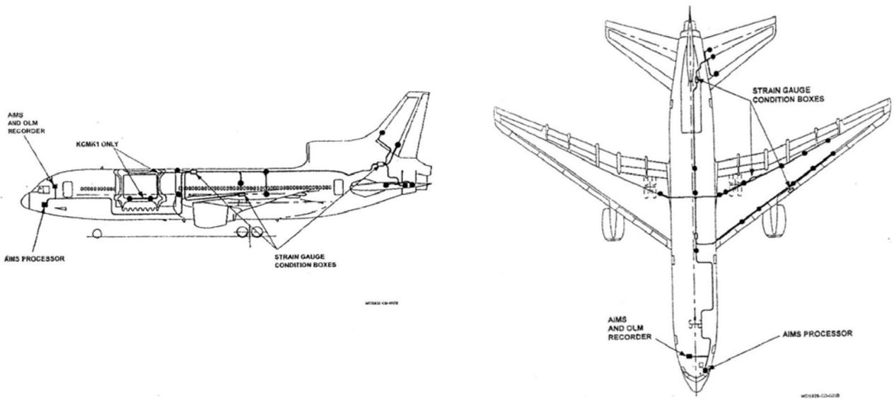
Figure 2-7 Strain Gauge Routing - Wing
