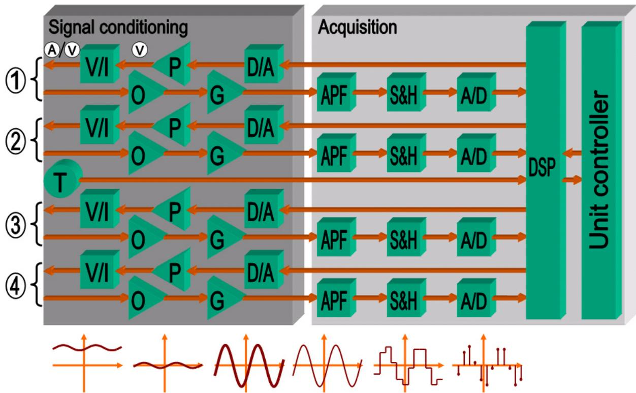
Figure 5: Sensor excitation, signal conditioning and processing inside Sensor-In module
