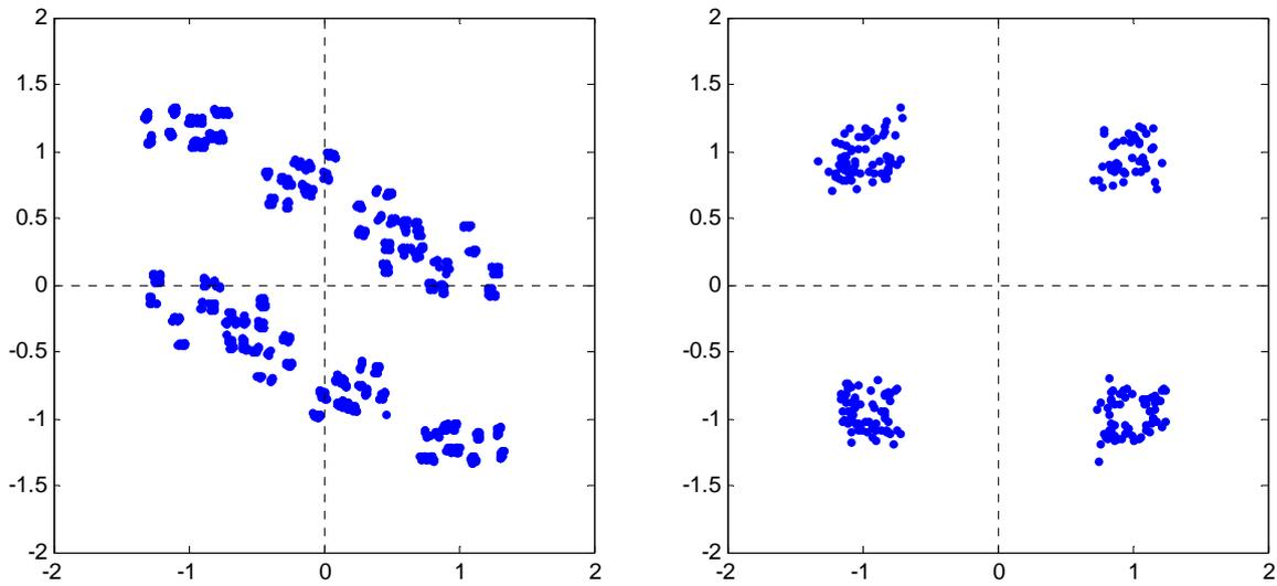
Figure 7: Performance improvement realized by the adaptive decision feedback MMSE equalizer applied to SOQPSK-TG transmitted over the channel with impulse response given by (7). The I/Q decision points without equalization are shown on the left. The decision points with equalization are shown on the right. The equalizer consisted of 21 feed forward coefficients, 18 feedback coefficients and used a step size of 0.001.
