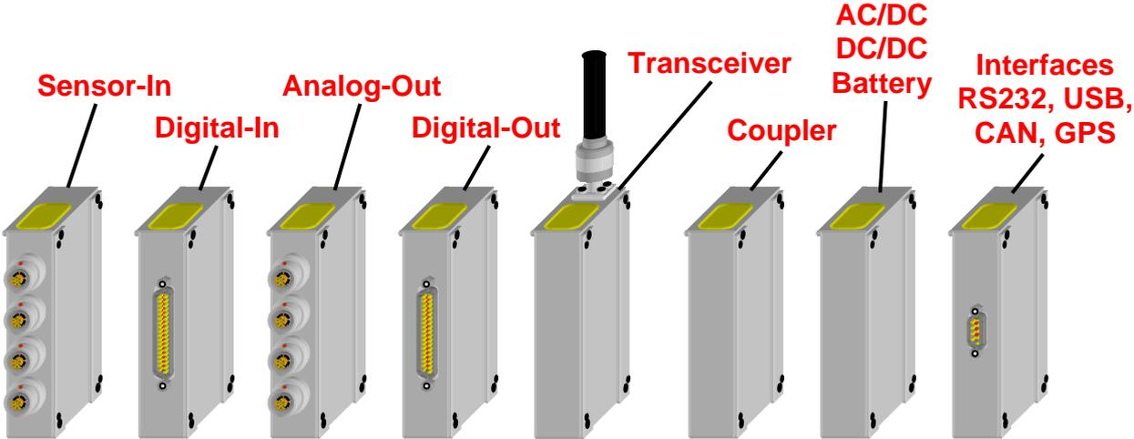
Figure 1: The modular structure of the system
