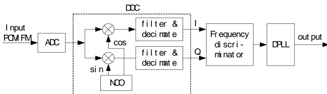
Fig.2 Block diagram of PCM/FM digital receiver
