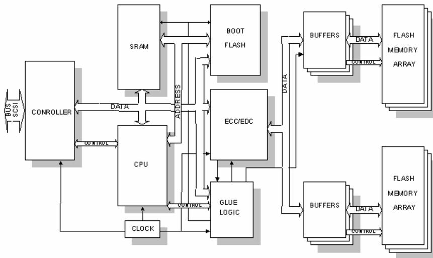
*Figure 1: Solid-state flash disk based on SCSI or ATA controller, Error Detection and Correction Code and a CPU, enabling the disk read/write operations to the flash array.*
