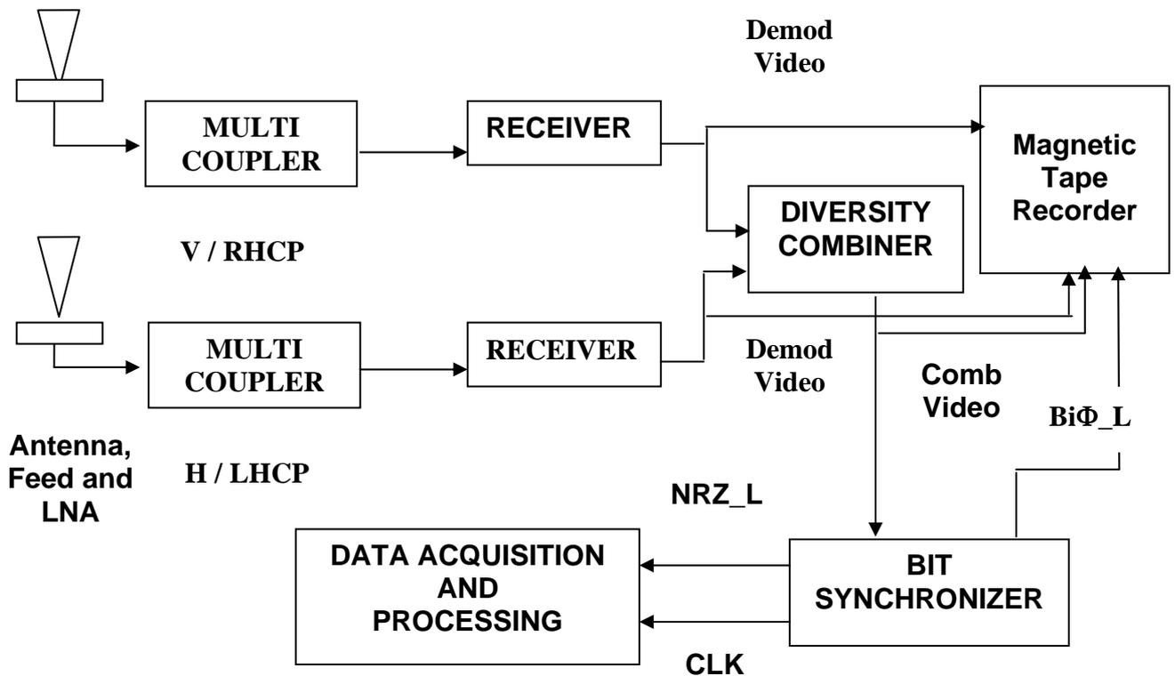
**Fig.1.0 : Typical Telemetry Ground Receiving Chain**
