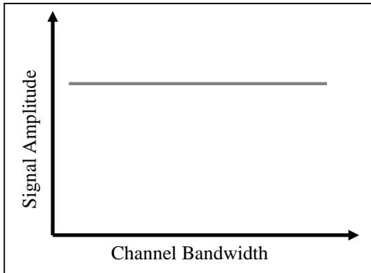
Fig. 2. Response of an Ideal Transmission Channel
