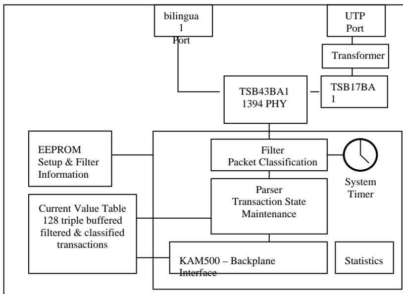
**Figure 4: ACRA CONTROL FireWire Bus Monitor**
