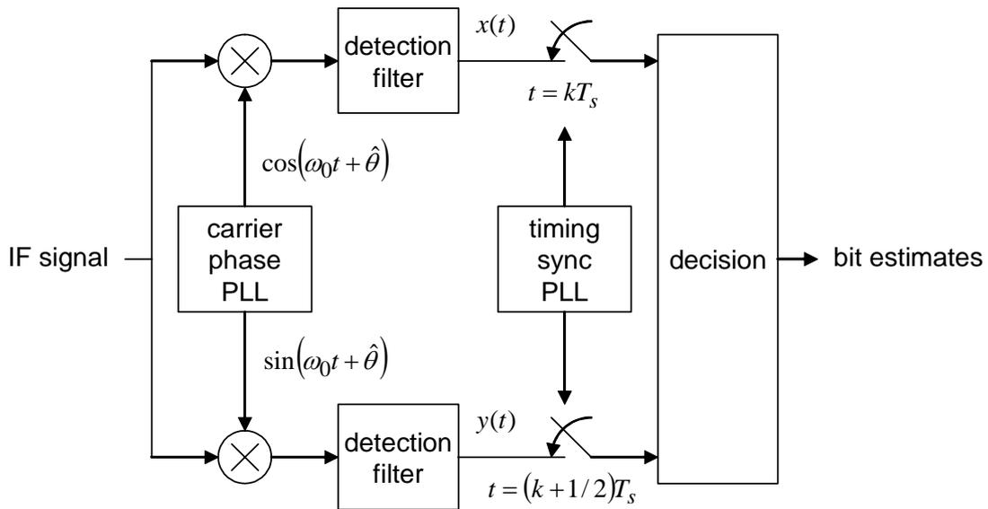
Figure 2: Generic detector for offset QPSK. This detector can also be used for symbol-by-symbol detection of FQPSK and SOQPSK.
