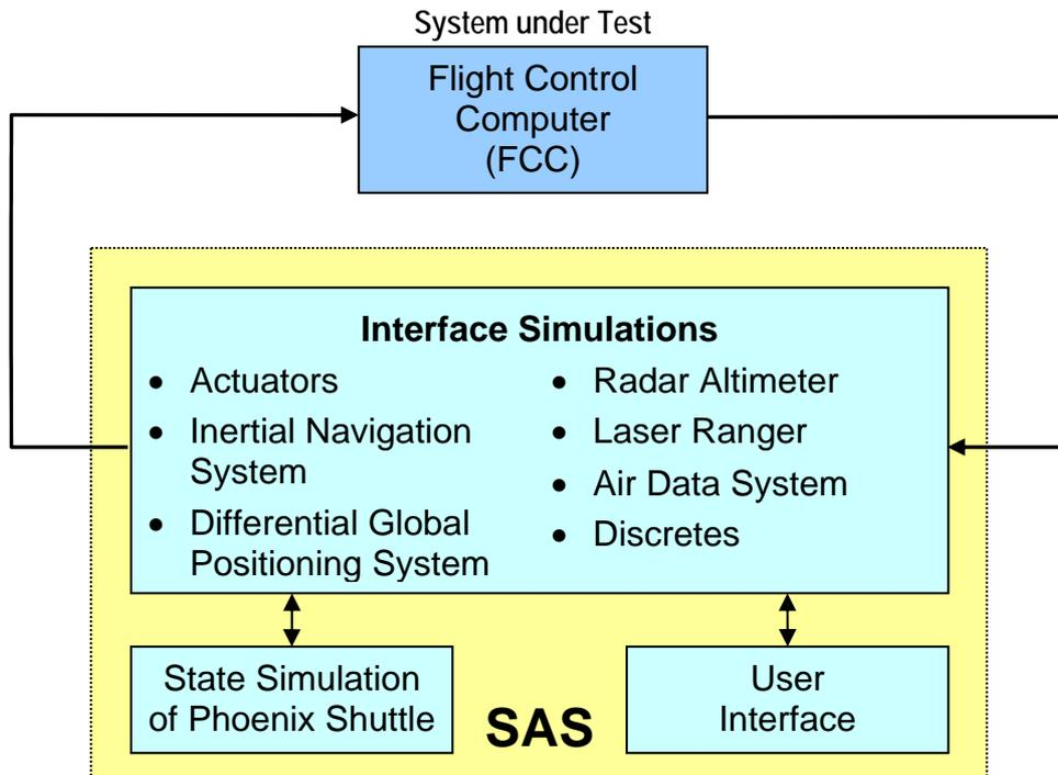
*Fig. 3: Hardware-in-the-Loop Principle*
