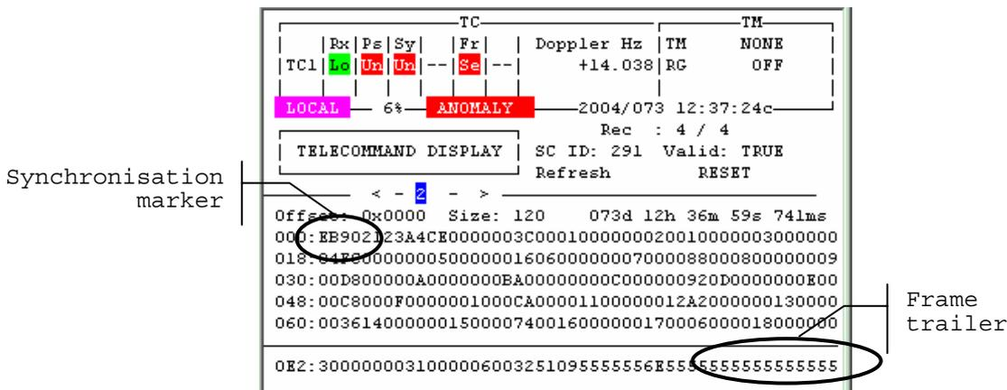
**Figure 4 : the HMI page for one extracted CLTU**
