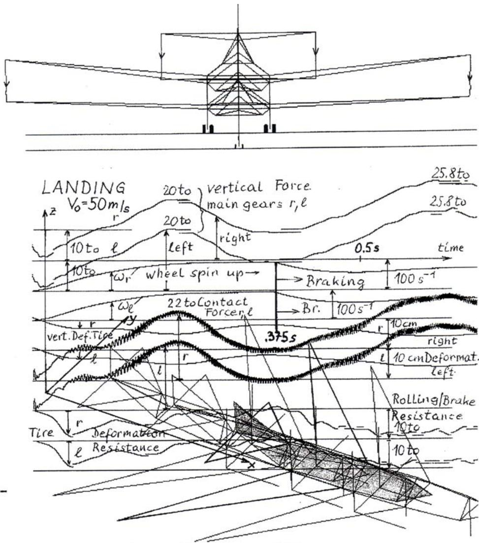
Fig.8 The landing is quite good a symmetric one but not exact, despite the fact that all parameters are defined symmetric. During braking the forces don't reach 20 to, the tire rotations aren't constant. On top animation is shown.
