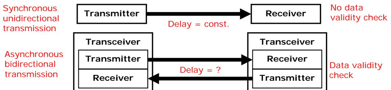
Figure 7: The two types of wireless data transmission
