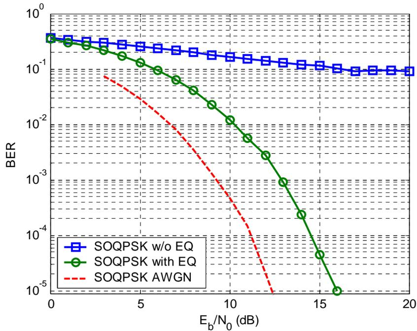
Figure 8: Bit error rate performance of 20 Mbit/sec SOQPSK-TG operating in a multipath channel with impulse response (7). The bit error rates with and without equalization are shown. The bit error rate performance of SOQPSK in the AWGN channel is included for reference.
