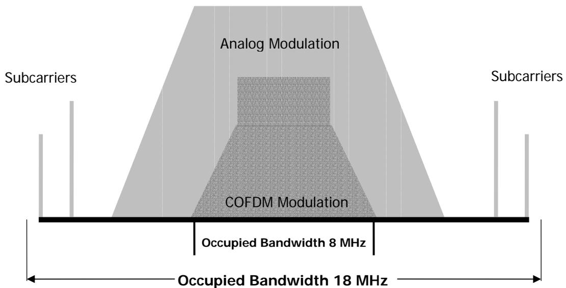
Fig. 6, Occupied Bandwidth of Analog and COFDM Digital
