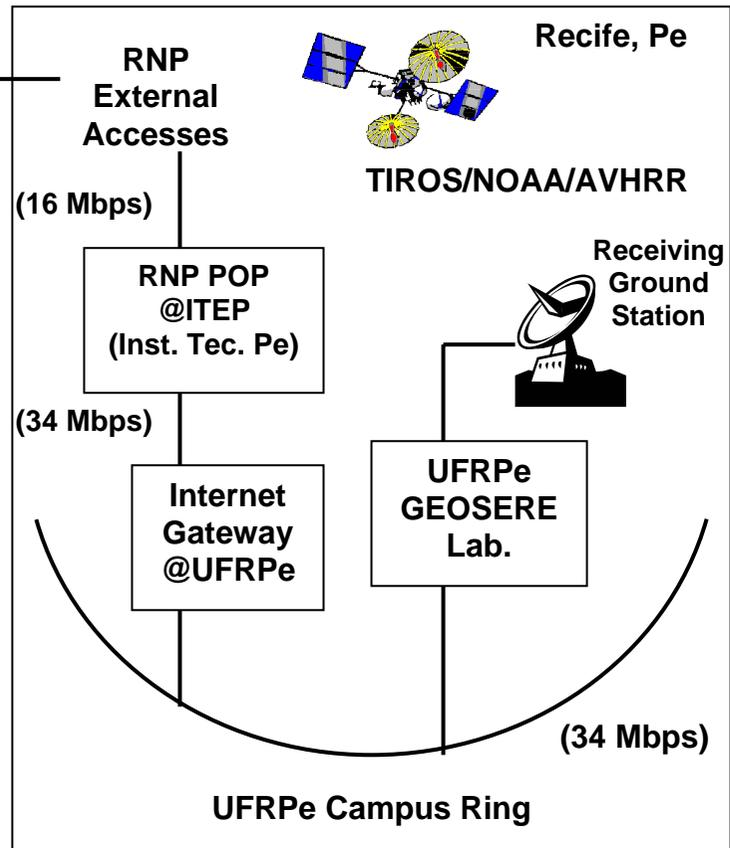
**Figure 2 - Relevant Details of Local Topologies**
