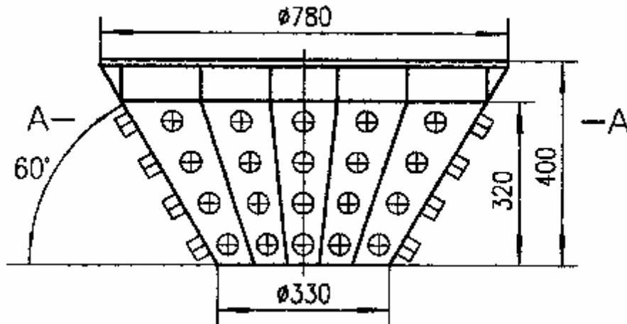
Figure 1 on-board phased array telemetering antenna structure
