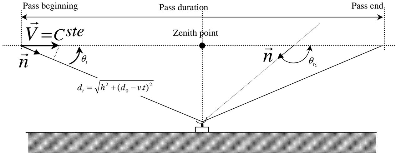
**Figure 6 : orbit model with a flat ground, constant altitude and constant speed**
