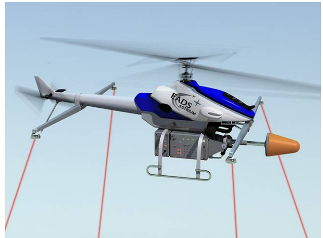
Figure 5: ANTF RC-Helicopter equipped with RF-Payload and Laser Targets
