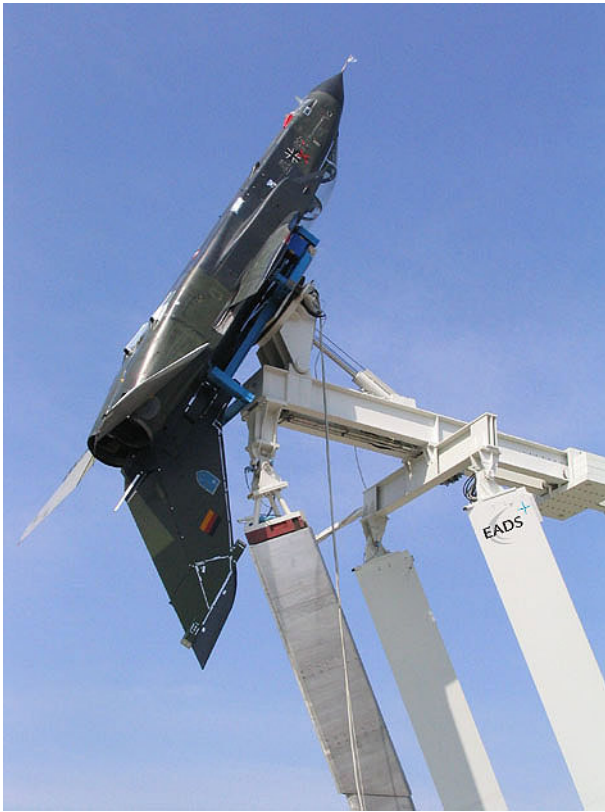
Figure 2: 'RaSigma' Positioner Set-Up for ARP Measurements of Full-size Aircraft Mock-Ups
