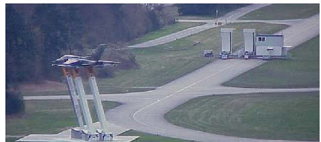
Figure 1: 'RaSigma' Far-field Range for Antenna & RCS Measurements; Set-Up for In-Service Aircrafts
