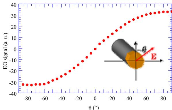
**Figure 3: Measured selectivity of a  $\text{LiTaO}_3$  probe to one component of the E-field.**
