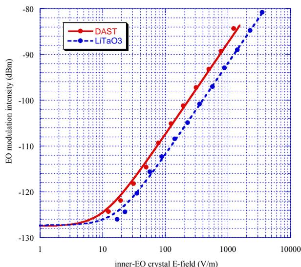
**Figure 2: Comparison between inner-crystal E-field responses of 10-GHz bandwidth  $\text{LiTaO}_3$  and DAST probes measured using a spectrum analyzer at 612 kHz with a 30-Hz resolution bandwidth.**
