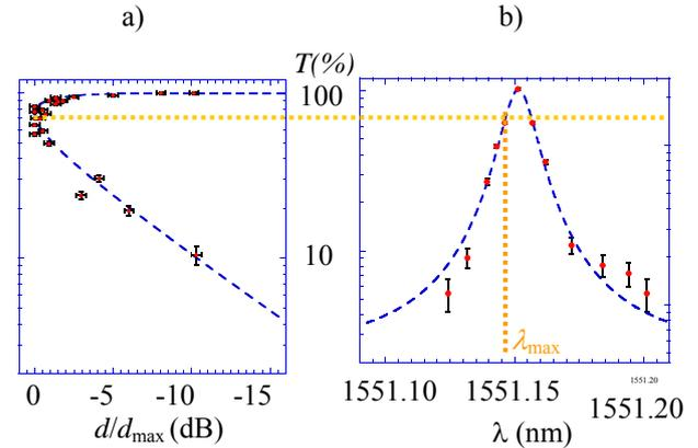
**Figure 5: Measured and theoretical transmission of the cavity (b) and associated normalized modulation depth (a).**
