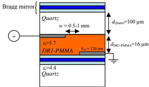
**Figure 4: Schematic of the realized organic EO microcavity**
