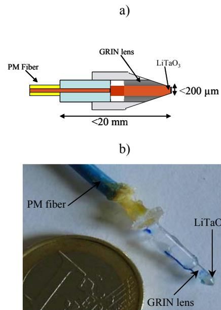
Figure 1: Schematic (a) and picture (b) of a fully dielectric conic-shape EO sensor.
