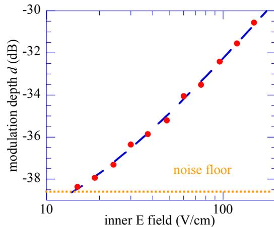
**Figure 6: Response of the cavity to electric field measured @ 500 kHz with a 30 Hz resolution bandwidth: experimental data (dots) and theoretical fit (dash line).**
