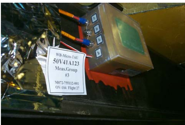
Figure 5 : WideBand MicroTAU Bonded to Shuttle
